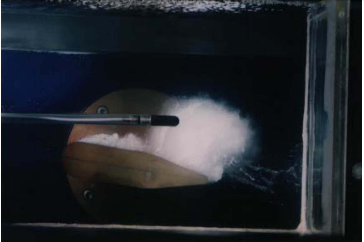
Fig. 6.3: Cavity appearance, KT section, 8^\circ , 12 m/sec., \sigma_B = 1.25
