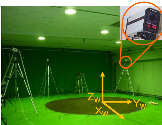
Fig.4. Motion capture systems (ProReflex TM MCU-500 + , Qualisys, Sweden).
